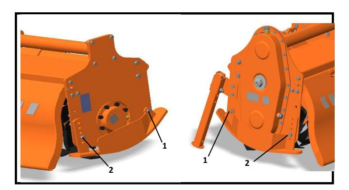
When finished, verify that both skids are at same level, and check if the front of the tiller is leveled to the back, when lowered to the ground. Adjust with the 3-point top link if necessary.
