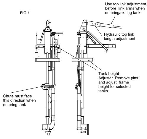
On entering the slurry tank ,use the hydraulic top link adjustment first. When the ram has reached the end of its stroke,you can then use the lower link arms to lower the slurry pump into tank if required.
