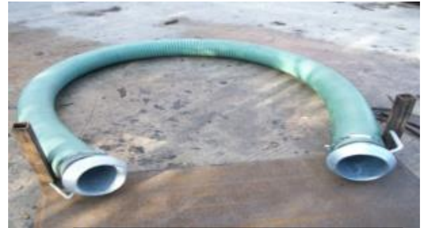
Fill pipe with identical ends connected to fill points of separate tankers, used to empty tanker that needs wheel changed.
