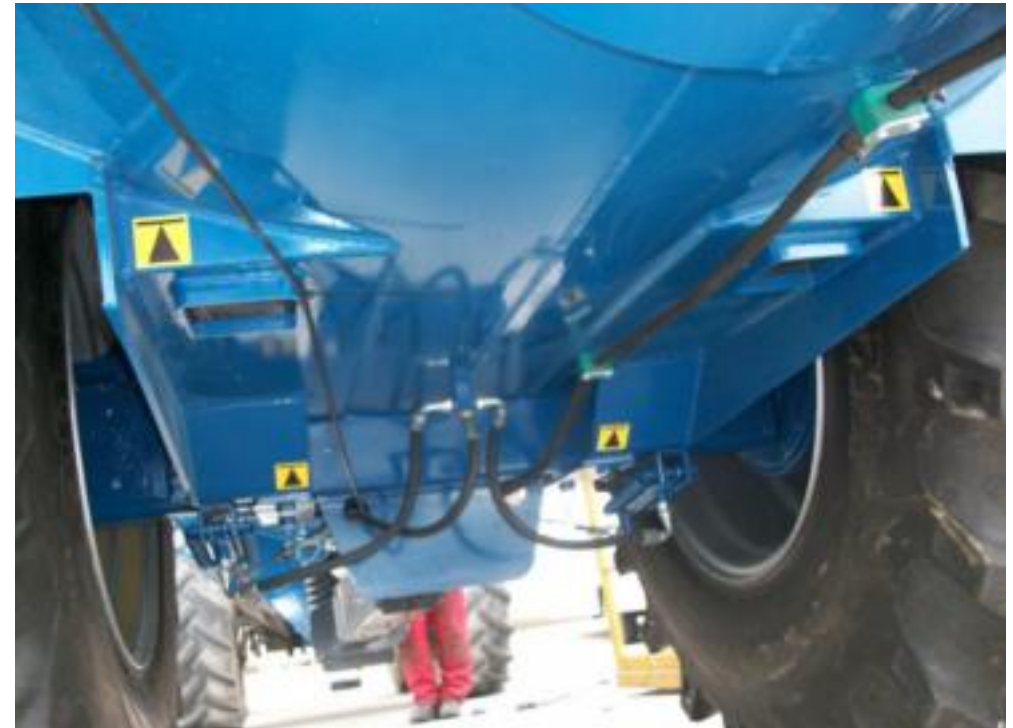
Locations of jacking points are clearly labelled at the back of the tanker.
