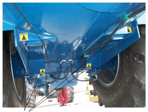
Locations of jacking points are clearly labelled at the back of the tanker.
