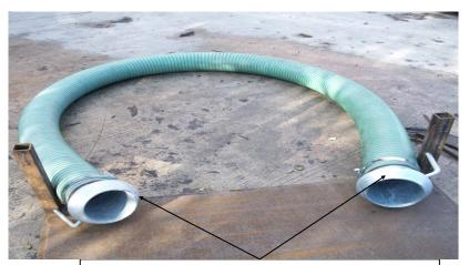
Fill pipe with identical ends connected to fill points of separate tankers, used to empty tanker that needs wheel changed.
