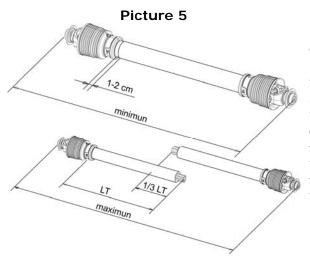
Check out that the cardan shaft minimum and maximum length are the ones required by the machinetractor coupling.
